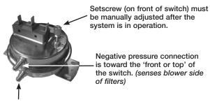
Positive pressure connection is toward the 'back or bottom' of the switch. (senses air inlet side of filters)
